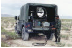
The Fibertek SR-BSDS uses the laser-induced fluorescence principle for BW agent detection.
