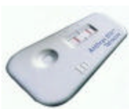
Tetracore Guardian BTA ('Bio Threat Alert ') test strips are agent-specific colorimetric testers using a colloidal gold immunoassay process.
